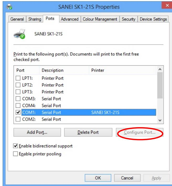
6-4. Unite a setup of a serial port and click "OK."
